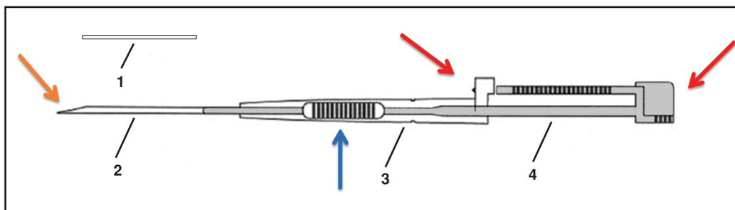
**Figure 2** Affordances present in the Implanon<sup>®</sup> applicator. Key: 1, Implanon rod; 2, needle; 3, plastic body; 2+3, cannula; 4, obturator. See text for an explanation of the significance of the coloured arrows. Figure modified from Mascarenhas L, Insertion and removal of Implanon<sup>®</sup>. *Contraception* 1998; 58(Suppl. 6): 79S–83S. © Elsevier, reprinted with permission
